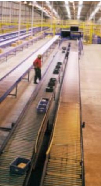
The North Island DC, covering some 580,000 sq. ft. is fully mechanised and automated. TallShips worked closely with Colby, who installed the accumulation conveyor and high-speed sorter, to ensure the WMS would handle both current and future stock volumes.
